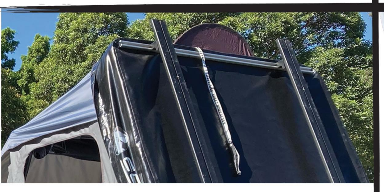
Roof Rails built-in to top for mounting roof bars or other accessories
